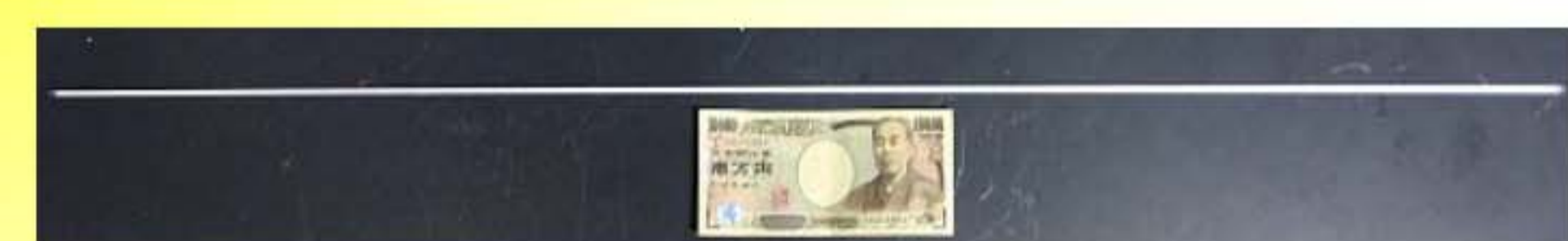
Fig 8 : 1m long DHEL (before lighting)
