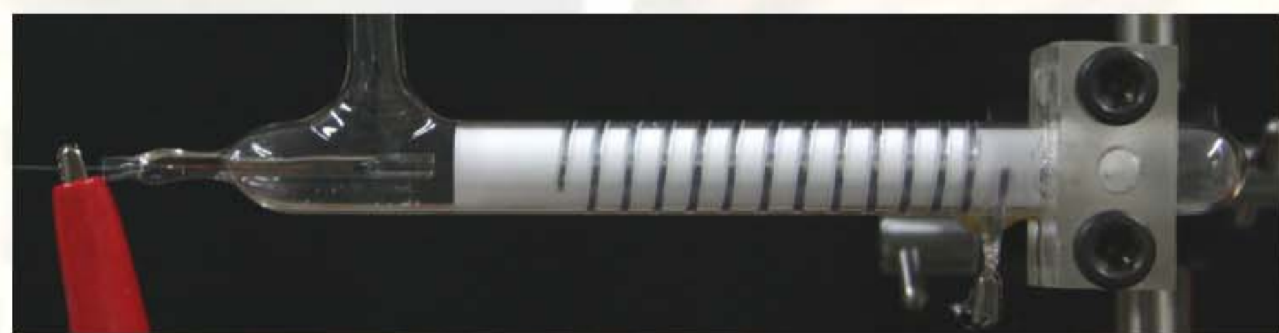
Fig.1. The discharge lamp (The phosphor is applied.)
