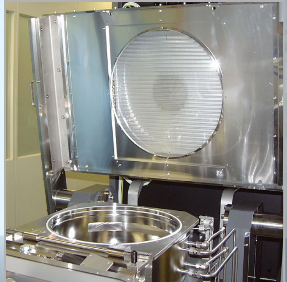
FLA machine for 12 inch wafer (Courtesy of Dainippon Screen MFG.,Co.,Ltd)
